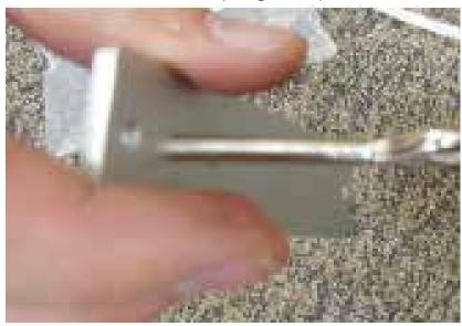
Clamp the belt brackets to the frame in such a way that the eye bolt will be in-line with the pulley on the back of the motor box.
