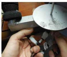
Run the network style cable with the display cable to the motor box.
