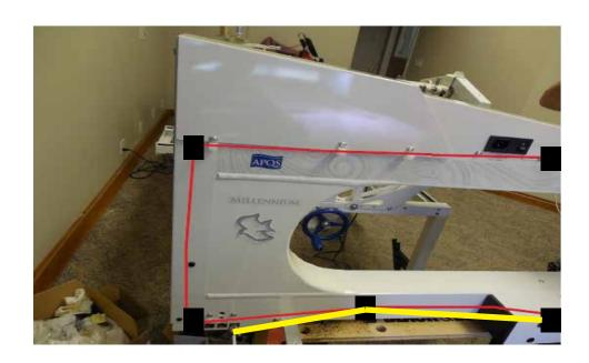
Run the handlebar cable to black motor box along side the display cable.
