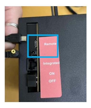
First plug in the Butler DC charging cable into the circle port on the robot.
