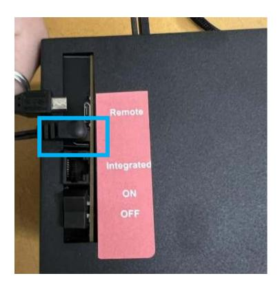
Next plug in the micro USB port (that is on the same side of the cable as the Butler DC charging cable) into the micro USB port on the robot.
