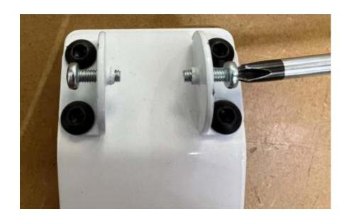
Align the holes in the display clamp with the holes in the display bases. You may need more than one person for this step.
