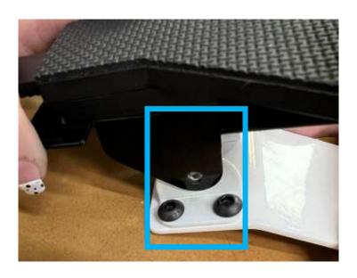
Screw the screws back into the bracket.
