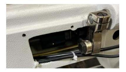
Next locate the a white cover that is located just above your motor. There are 7 screws that need to be unscrews and saved for later. There will also be cables in this part of the machine when you take off the cover.
