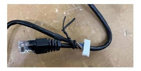
Once you have finished this your are going to go back to the front of the machine and take the cable that you pulled out of the display earlier and then pull the cable through until the new cable with the RJ45 (phone cable end) is pulled through far enough to connect to your display.
