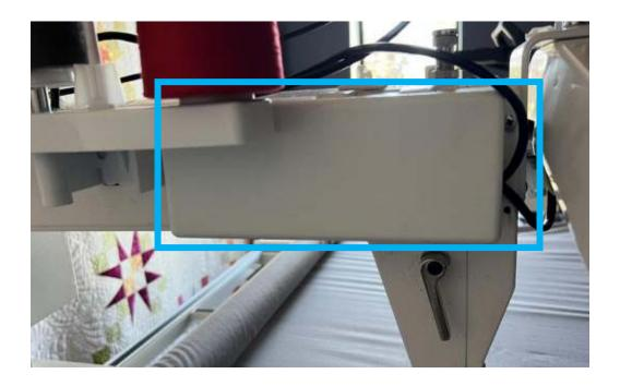
The second way is if your machine does not have a side port under the rocker arm cover.The rocker arm cover is the rectangular cover on the front, left side of the machine (if you are facing the front of the machine) just in front of the thread stand.
