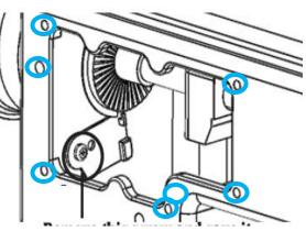
Once that is open we are going to want to locate the white or black box on the rear of your machine. This is the box the power cable plugs into. <u>MAKE SURE TO UNPLUG THE</u> <u>POWER CABLE BEFORE YOU DO ANYTHING</u> <u>WITH THIS BOX.</u> There are 4 screws that you will need to unscrew and save for later.
