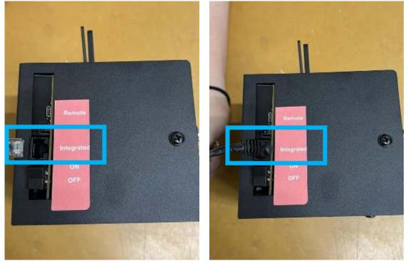
Run the other end of the Ethernet cable along side your machine and then plug it into the robotics port on the white or black box of your long arm machine. (If you are looking at the front of your machine, the white or black box is on the right side at the back of your machine, it is where the power cable plugs in.)
