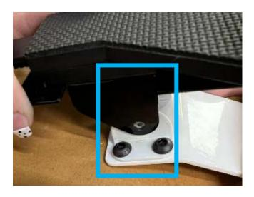
Screw the screws back into the bracket.
