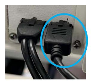
Next you are going to want to take the external remote cable and plug the black 10 pin side into the port that you just removed the old cable from.
