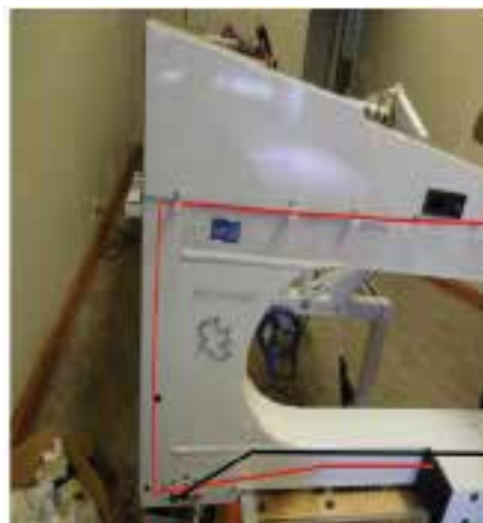
Pictured APQS machine; display cable show in red
