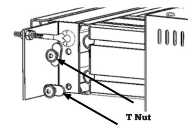
Attach Belt Bracket to T-nuts and tighten securely using provided screws.
