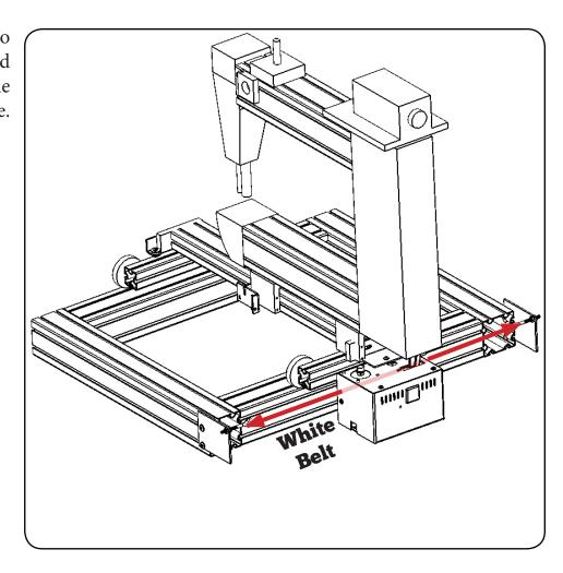
Make sure that the teeth side of the belt are facing the motor box pulley.
