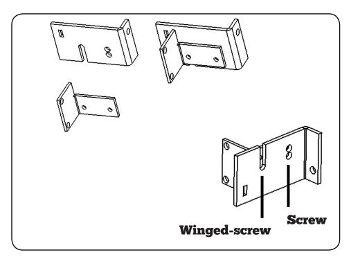
Attach the carriage bracket to the frame as indicated at right using the provided screws.
