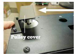
Tighten nuts onto top of screws to secure the Pulley cover.
