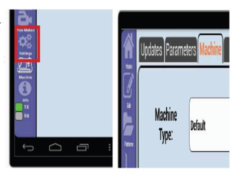
2 Select the Machine Type dropdown and select the proper machine type.
