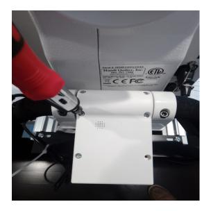
Remove the rear cover and unplug the 2 handle bar cables.
