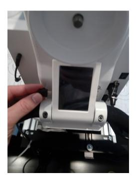
Pivot the display away from the machine and remove the 6 screws from the back of the display.
