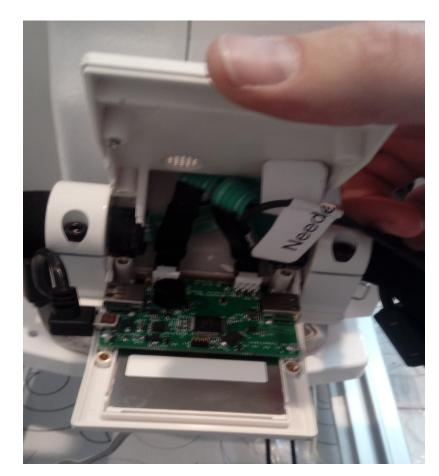
Route the robotics "handle bar" wire through one of the side USB ports.
