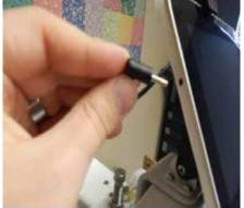
5 Locate display cable. It will be a network style cable on one or both ends.
