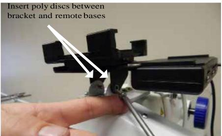
Images used are not representative of all display brackets. Use these concepts to mount the remote bases to the provided display bracket.
