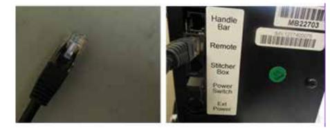
For Machines with QuiltEZ Electronics: Plug the remaining end of the black cable into the port near the front of the machine.
