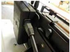
6 For Robotics Only: Plug the ethernet end of the black cable into the Remote port on the Black Motor Box
