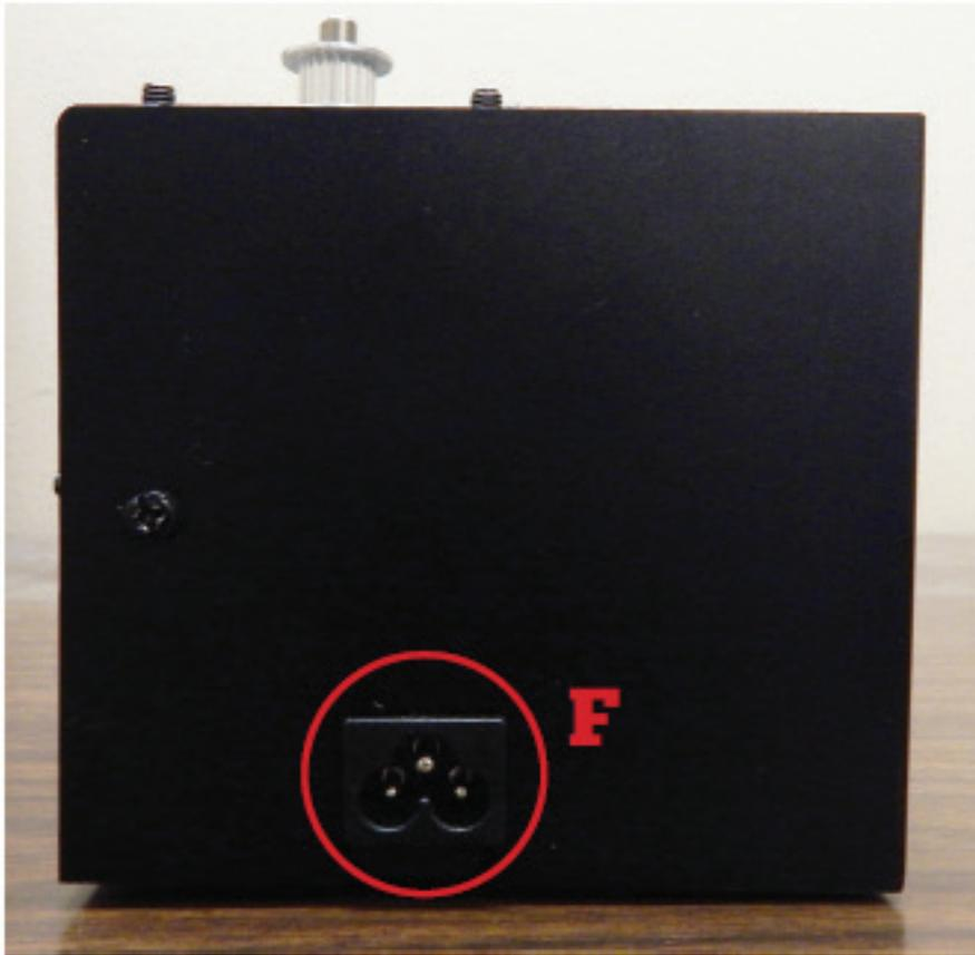
**F** On the opposite side is an internal power supply port. This is where the power cable gets connected to the robot.
