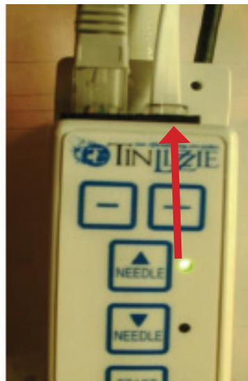
For RAM style handlebars (right) plug the other end of the cable into the center phone style plug (plug should be a 6 pin connection).
