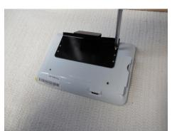
Loosen faceplate screws and slide display bracket tab between faceplate and machine head. Tighten faceplate screws.
