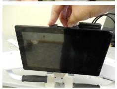
Lock clamps back in place and plug in wires to the DC IN and OTG ports.
