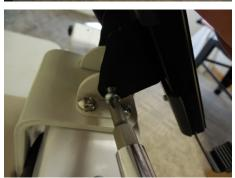
Unlock clamp from back of display holder and raise clamp.
