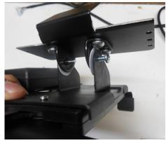
Loosen faceplate screws and slide display bracket tab between faceplate and machine head.
