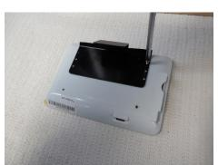
Loosen faceplate screws and slide display bracket tab between faceplate and machine head. Tighten faceplate screws.
